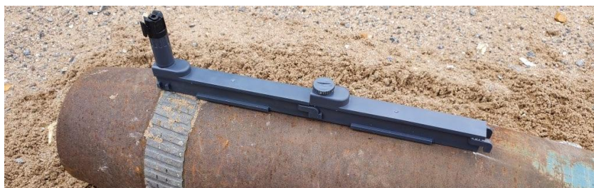
Figure 5 – Alford's Technologies Dioplex EOD (linear shaped charge) fitted onto UXO [10].
