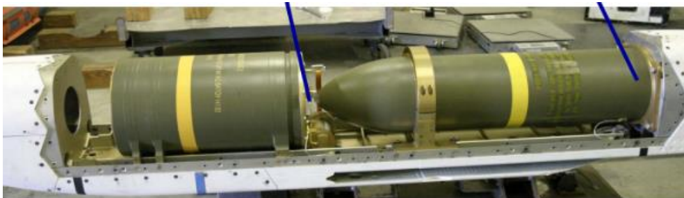
Figure 4 – Shaped charge and follow through bomb as used in AGM-154C [9].
