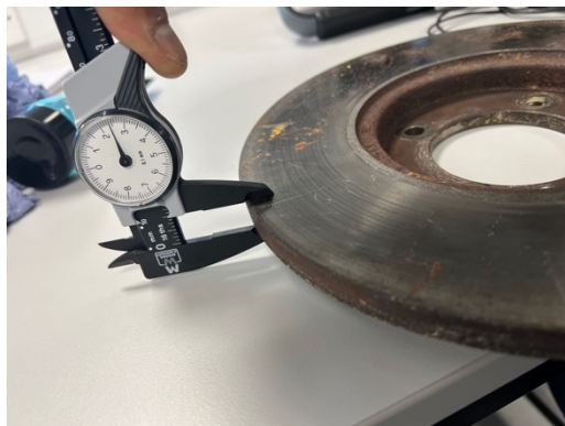
Figure 8: Thickness measurement of brake rotor
