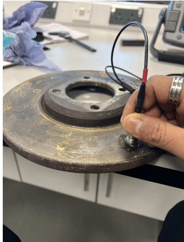
Figure 6: Apparatus connections for experiment for disc brake
