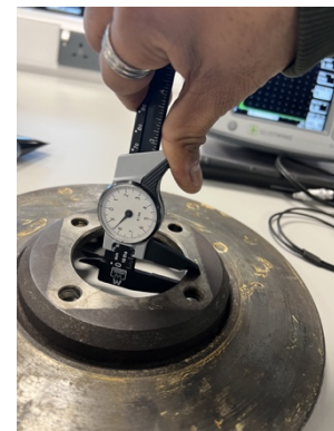
Figure 9: Thickness measurement of brake hub
