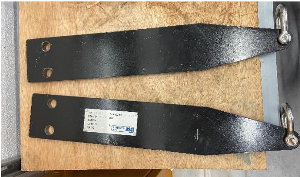
Figure 6 Calibration Arms of a known length.
