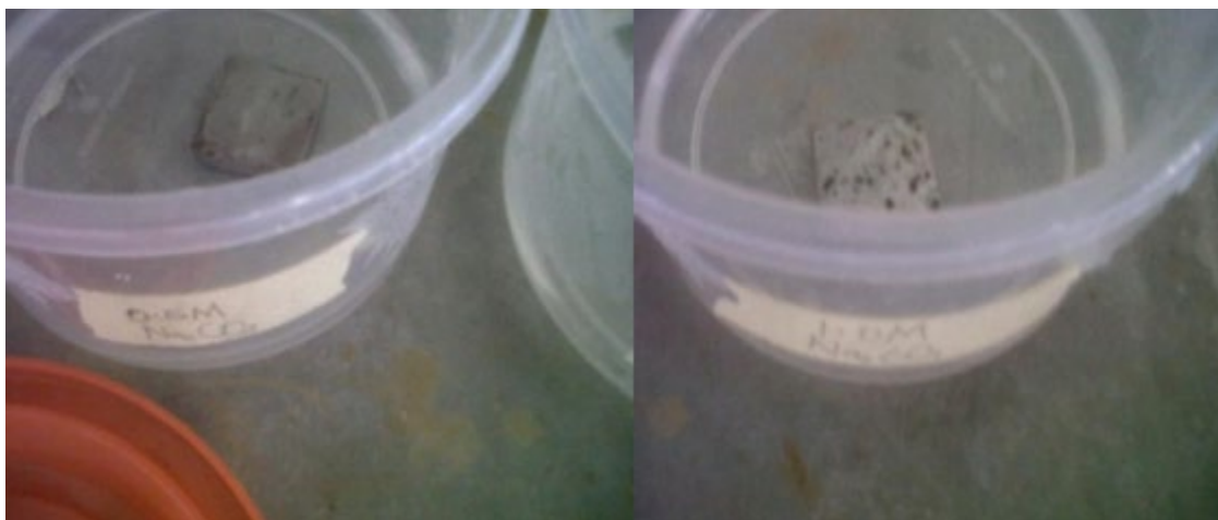
Figure 7: Immersed pieces of mild steel in 0.5M and 1M solution of \text{Na}_2\text{CO}_3
