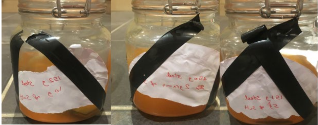
Figure 9: Colour changes in NaCl and distilled water at the end of 1008 hours
