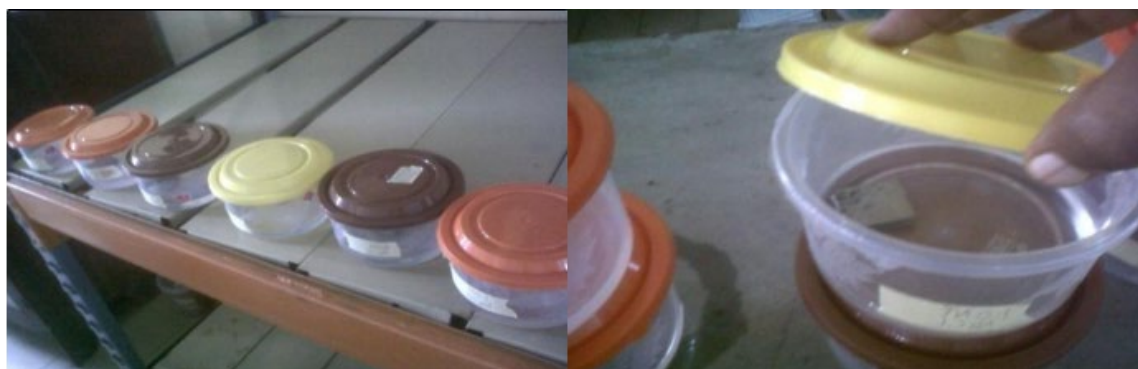
Figure 5: The setup of the immersion test
