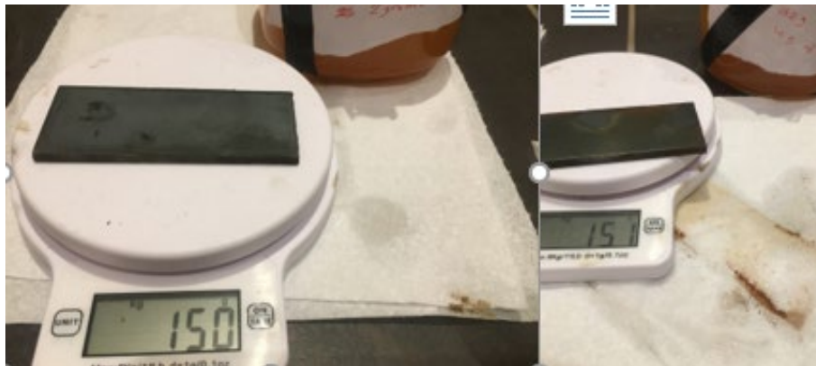
Figure 10: Change in weight of specimen dipped in 1M of NaCl solution after 7 days
