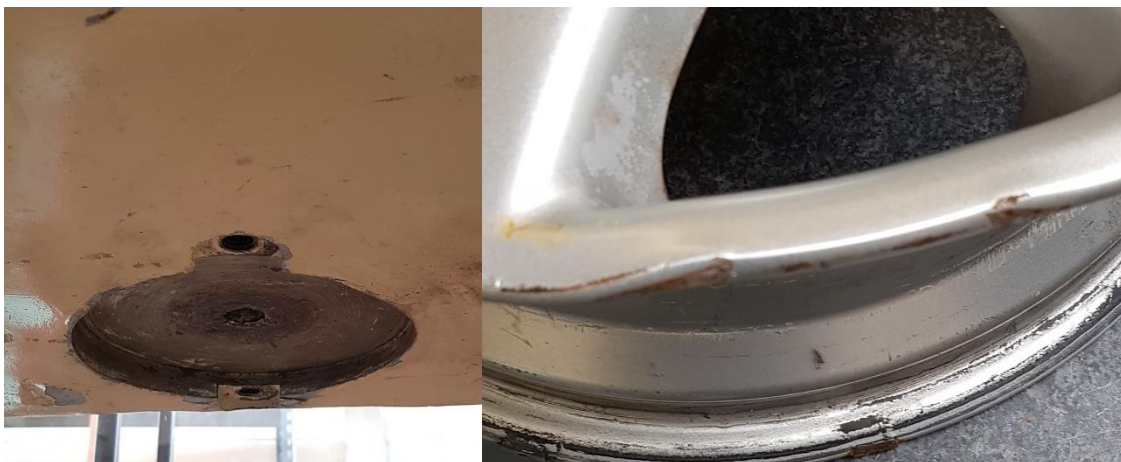
Figure 6.4 - Images showing the recess in the top plate and the damaged caused to Wheel 1
