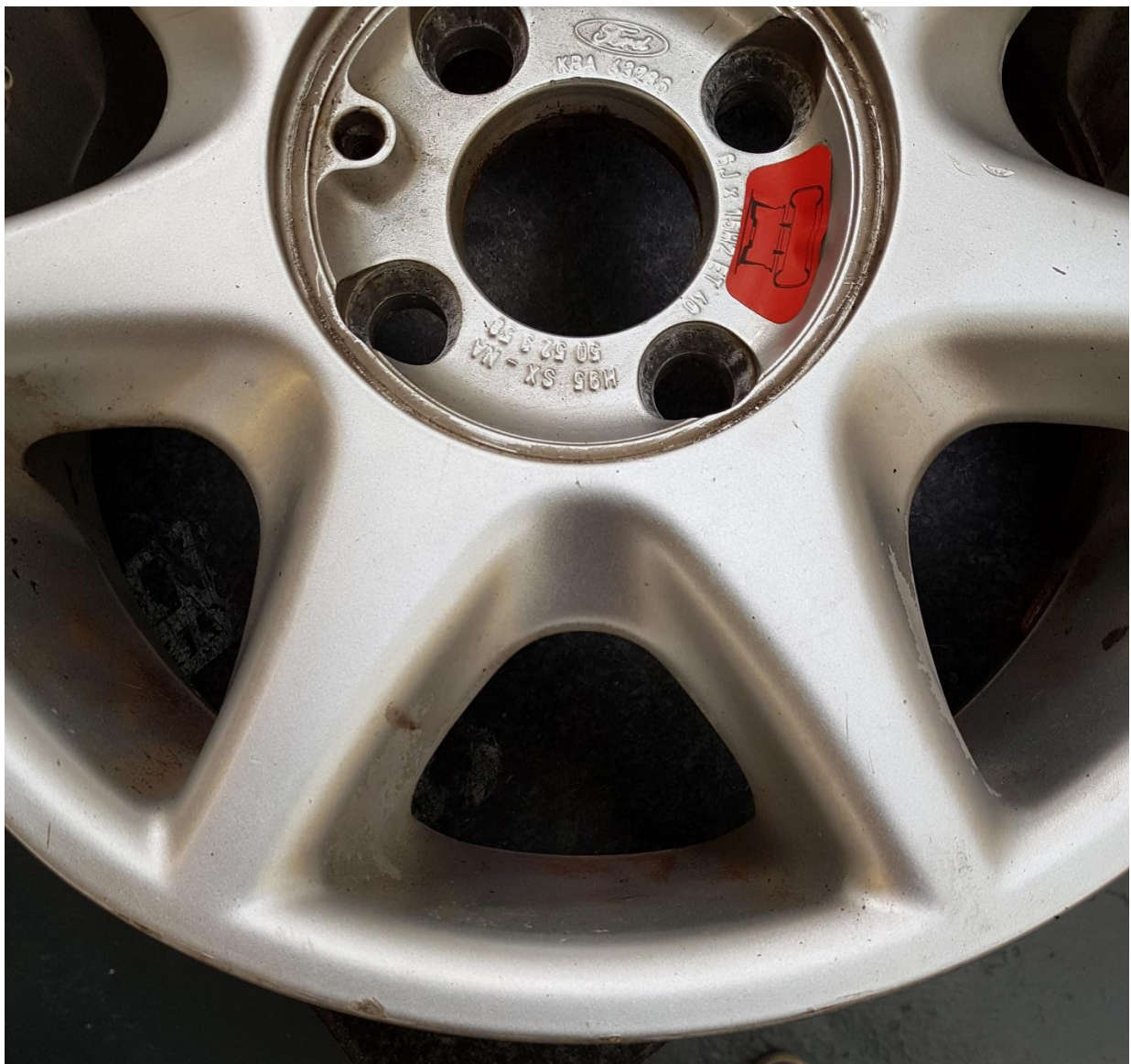
Figure 6.5 - Wheel 3 shows no sign of damage from the two runs
