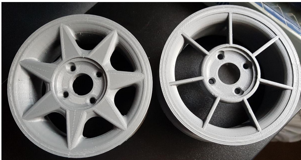
Figure 9.1 – Image showing 3D printed models and Ultimaker2 creating original model
