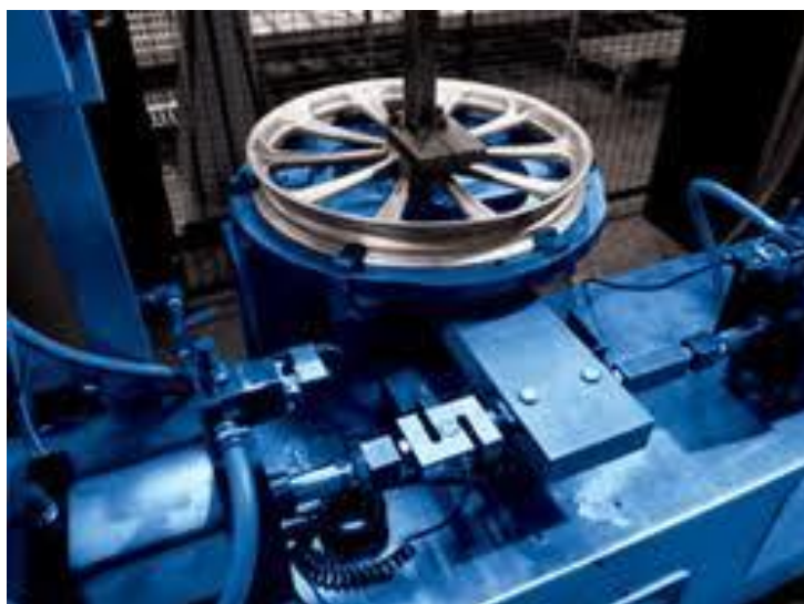
Figure 4.7 An image showing a torsional test (Performance Machine, 2018)
