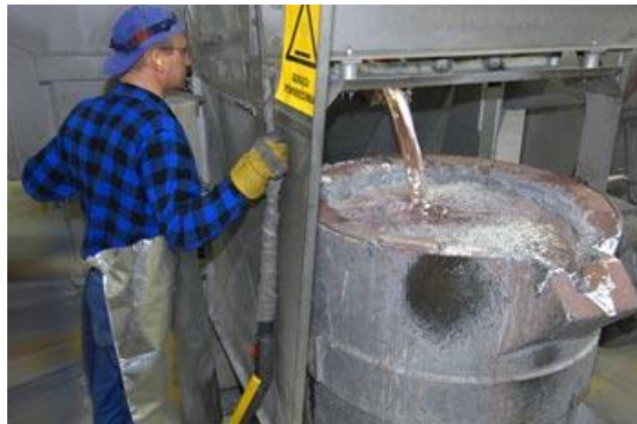
Figure 4.12 Casting an Alloy Wheel (Wolfrace, 2018)
