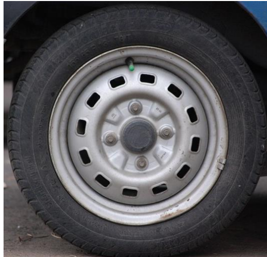
Figure 4.9 Example of a Steel Wheel (4FreeTextures, 2018)
