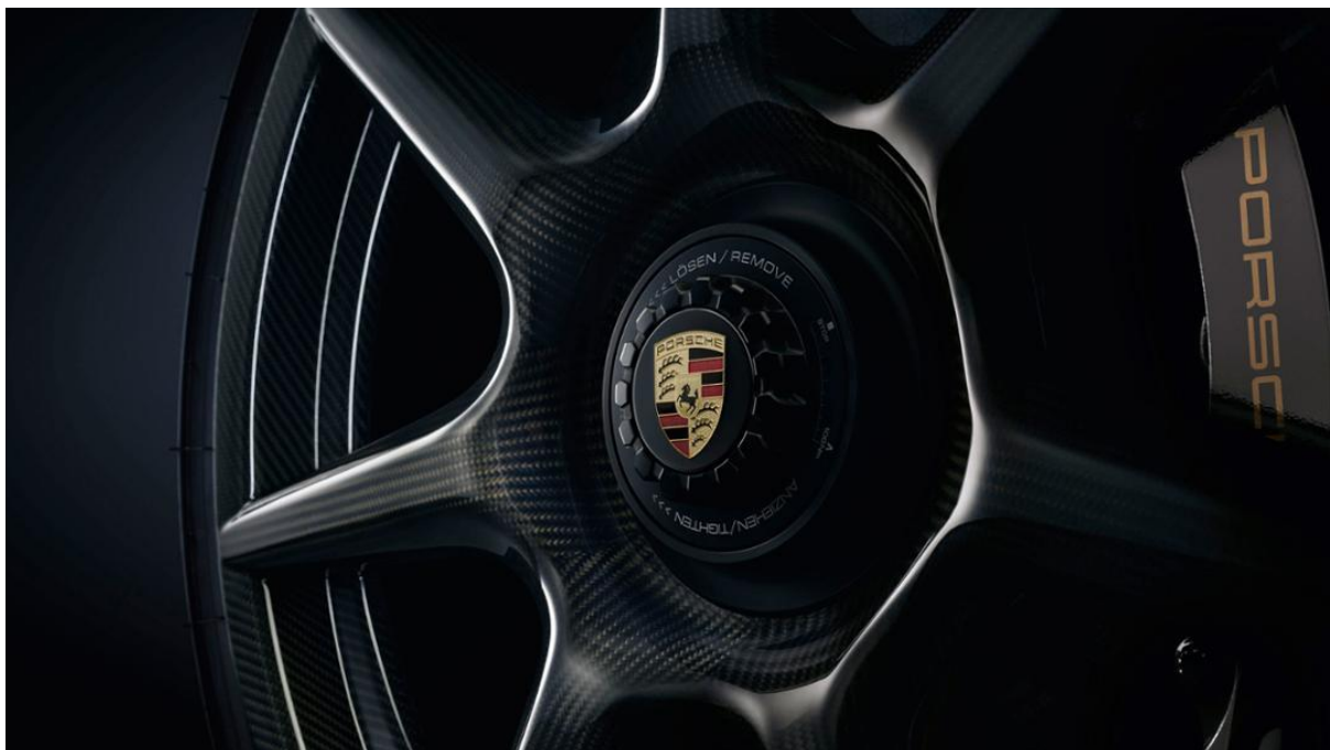
Figure 4.3 Porsche's Carbon Fibre Braided Wheel Porsche (2018)
