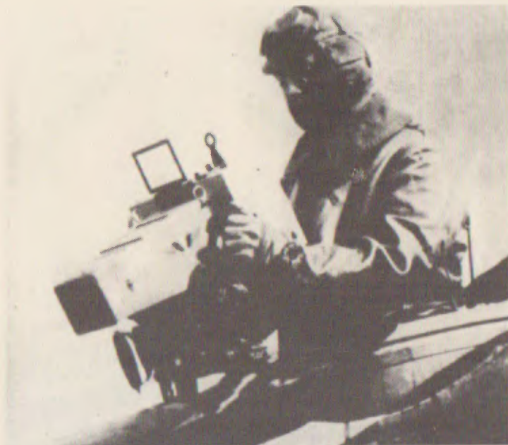
5. Camera mounted on a machine-gun emplacement, interfering with the aircraft's defences. The gun-grip is underneath the camera.
