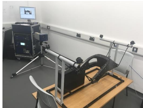
Figure13. LDV experiment - Swingarm
