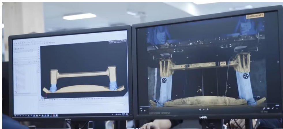
Figure 7. RIMAC FEA vs Physical Testing of system level
