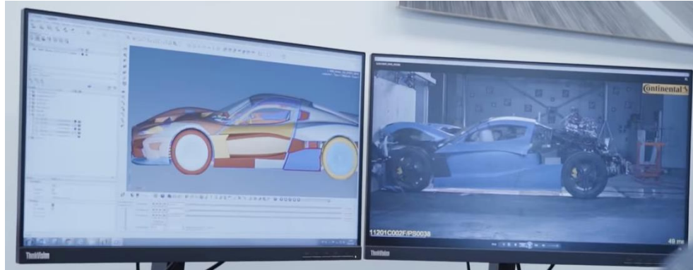
Figure 6. RIMAC FEA vs Physical Testing of full vehicle
