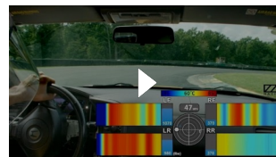
Overlay of Tire Temperature and Wheel Loads at VIR – Ize-Racing
