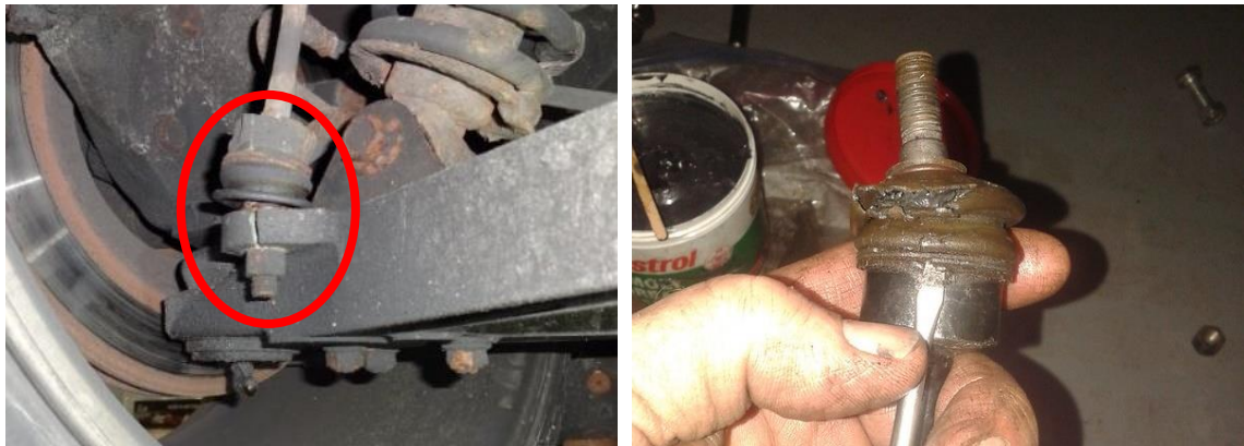
Figure 11 – Drop Link Fixture Fracture (Left), Drop Link Dust Cover (Gaiter) Failure (V10 SPM, fatboy18, 2016)
