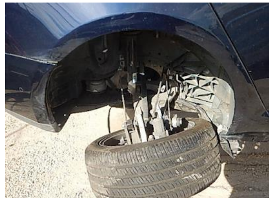
Figure 36 – Corrosion Display On The Chassis Of A Land Rover Defender (Left) (Glen Coyne, 2021), Tesla Model S Wishbone Failure (Right) (Wivaneff, 2016)
