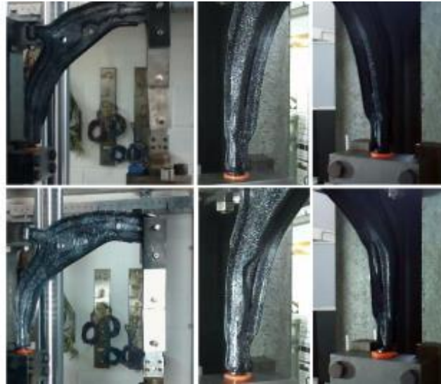
Figure 28 – Forced Displacement Of The Wishbone At 0mm (Top), 50mm (Bottom) (Farquharson-Laver, 2014)
