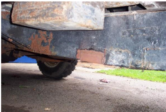
Figure 36 – Corrosion Display On The Chassis Of A Land Rover Defender (Left) (Glen Coyne, 2021), Tesla Model S Wishbone Failure (Right) (Wivaneff, 2016)
