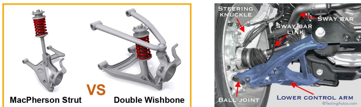
Figure 2 – MacPherson Strut vs Double Wishbone Suspension System (Left) (Stevens, 2020), Diagram Of Wishbone Connections (Right) (Testing Autos, 2020)
