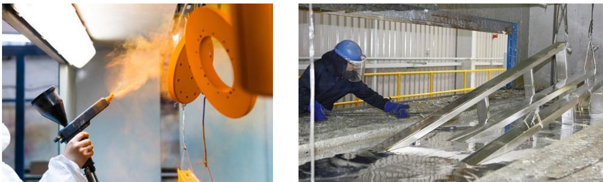
Figure 14 – Application Of Protective Coatings, Powder Coating (Left) (Ronquillo, 2021), Galvanising Steel (Right) (Sperrin Galvanisers, 2021)
