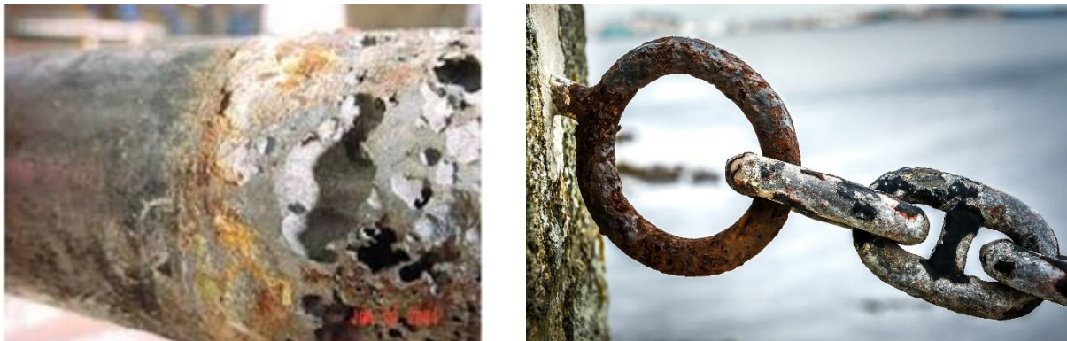
Figure 13 – Effect Of Salt Water Rusting Away Metals Containing Iron (Left) (Redazione, 2014), (Right) (Gillespie, 2018)
