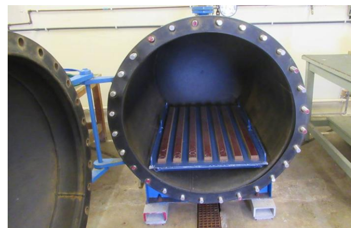
Figure 4 – Water pressure test chamber
