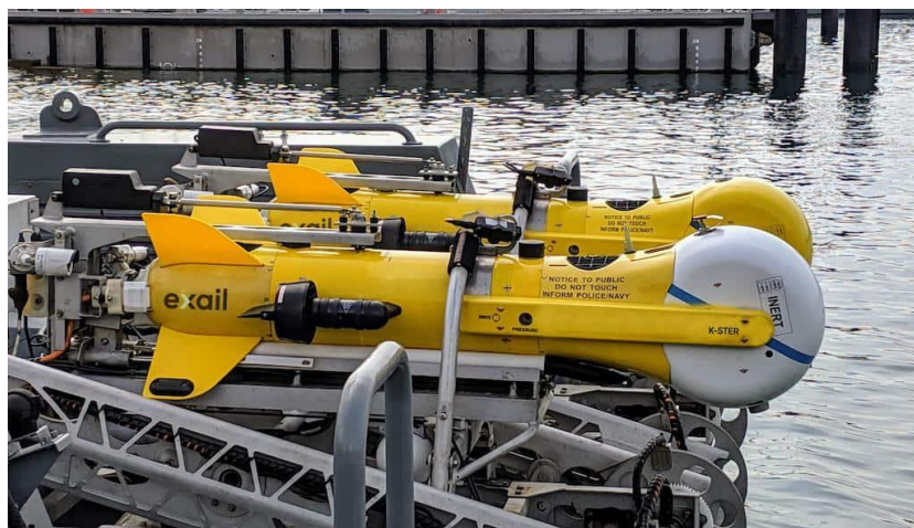
Figure 3- Exail K-Ster C Underwater EOD robot [4]
