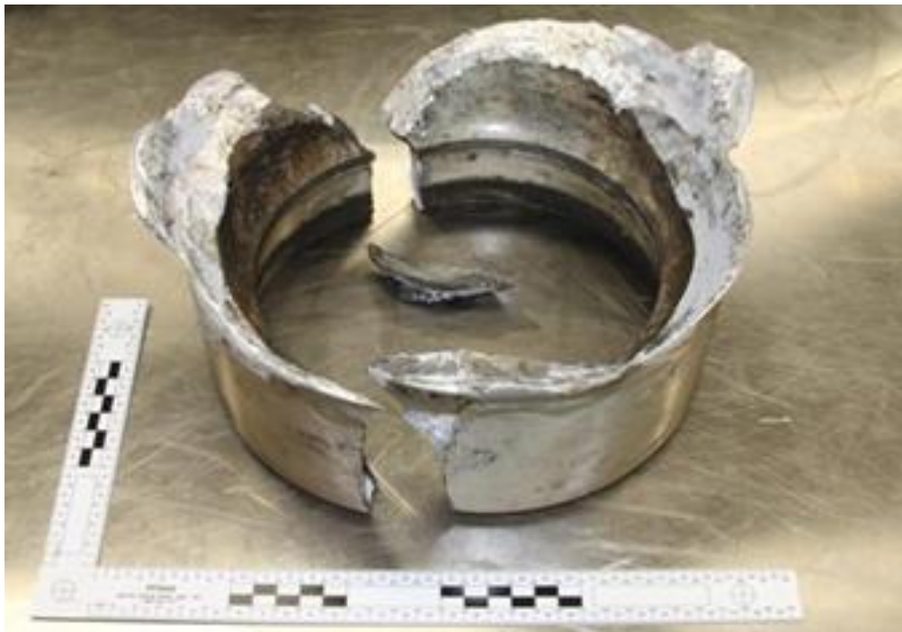
Figure 17 Fractured Hub Section [13]
