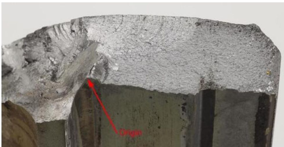
Figure 16 Crack Initiation at Bearing Bore Corner Radius
