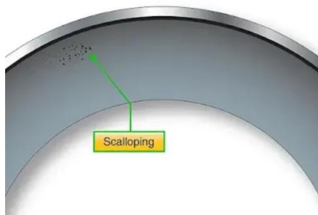
Figure 6 Scalloping, Eventually Leads to Wheel Bearing Failure [1]
