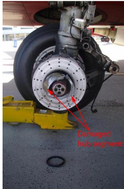
Figure 14 Exposed Wheel Bearing Fracture on Main Landing Gear Assembly [13]
