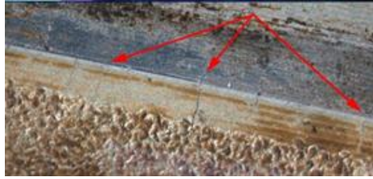
Figure 22 Radial/Axial Cracks Adjacent to the Shot-Peened Area (High Magnification) [13]
