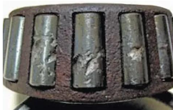
Figure 8 Spalling, Sub-surface Cracks Leads to Surface Fatigue [1]
