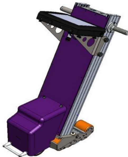
Figure 4: Example of MFL floor scanner inspection system ((Uk), 2017)
