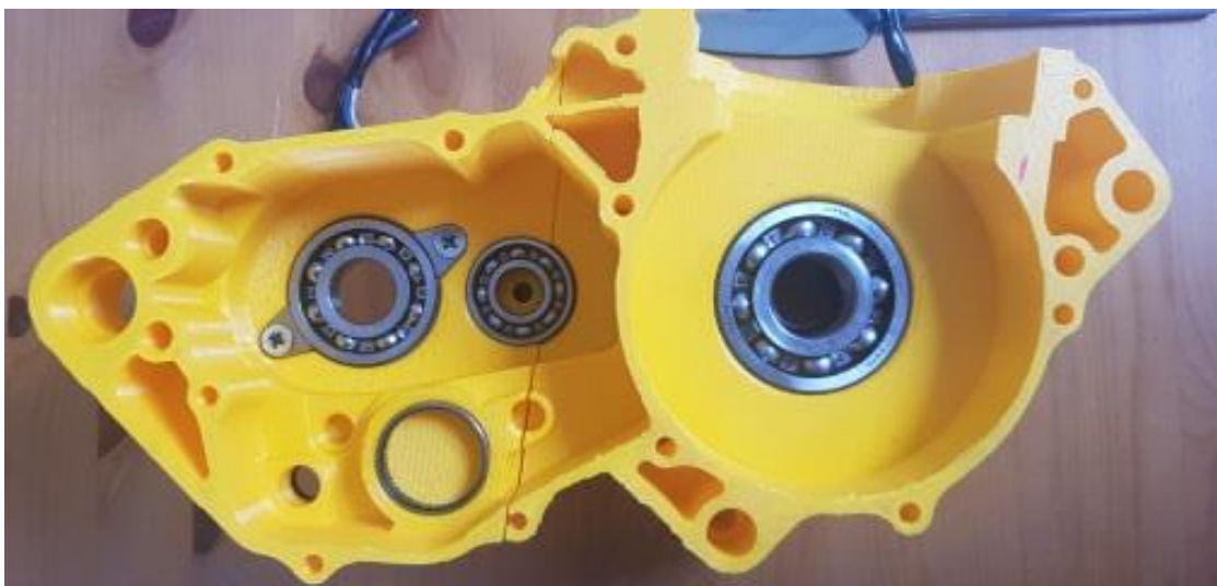
Figure 12 – Left-hand crank case fitted with all bearings, seals, stator plate and clutch slave cylinder. (Parsons, authors own)
