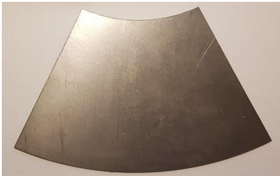
Figure 32 – Truncated cone section used in straight sections where there is an increase in diameter but no change in direction. (Parsons, authors own)
