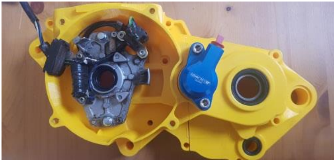
Figure 11 - 3D printed generator cover. (Parsons, authors own)
