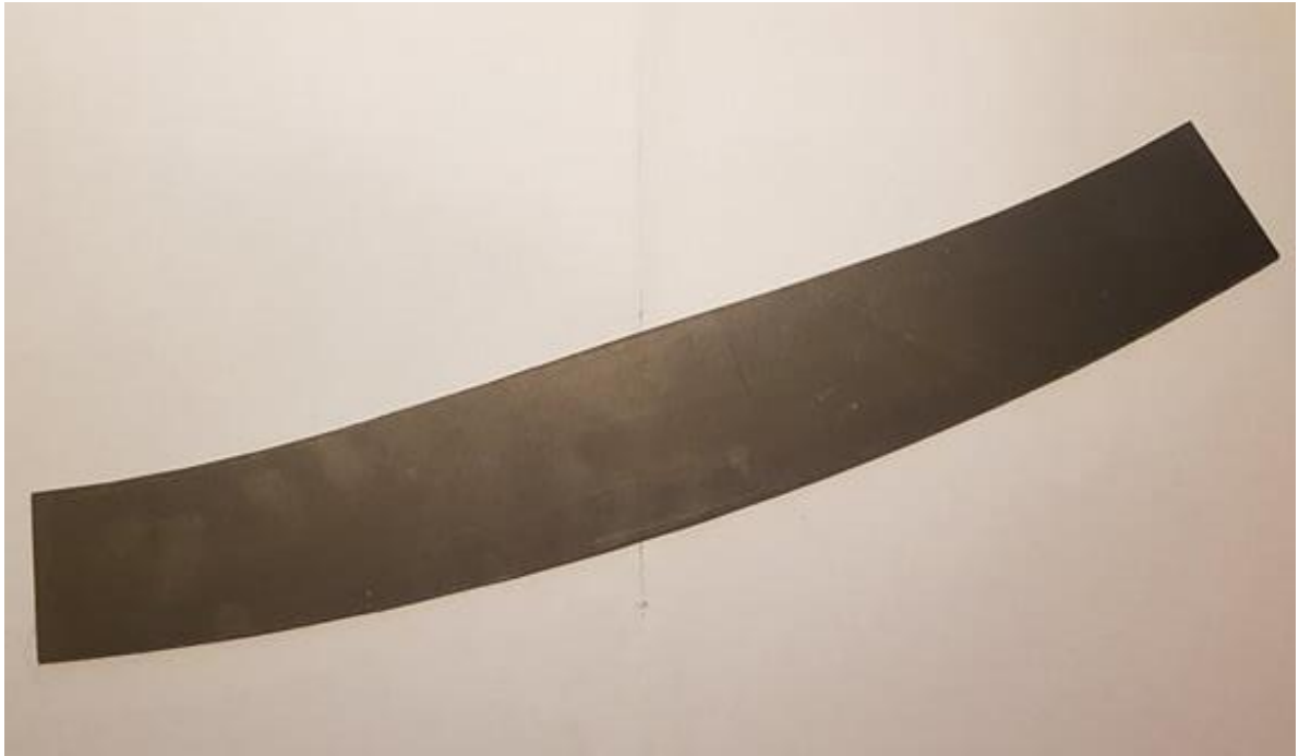
Figure 34 – Truncated Cone with angled top, waterjet cut from mild steel sheet. (Parsons, authors own)
