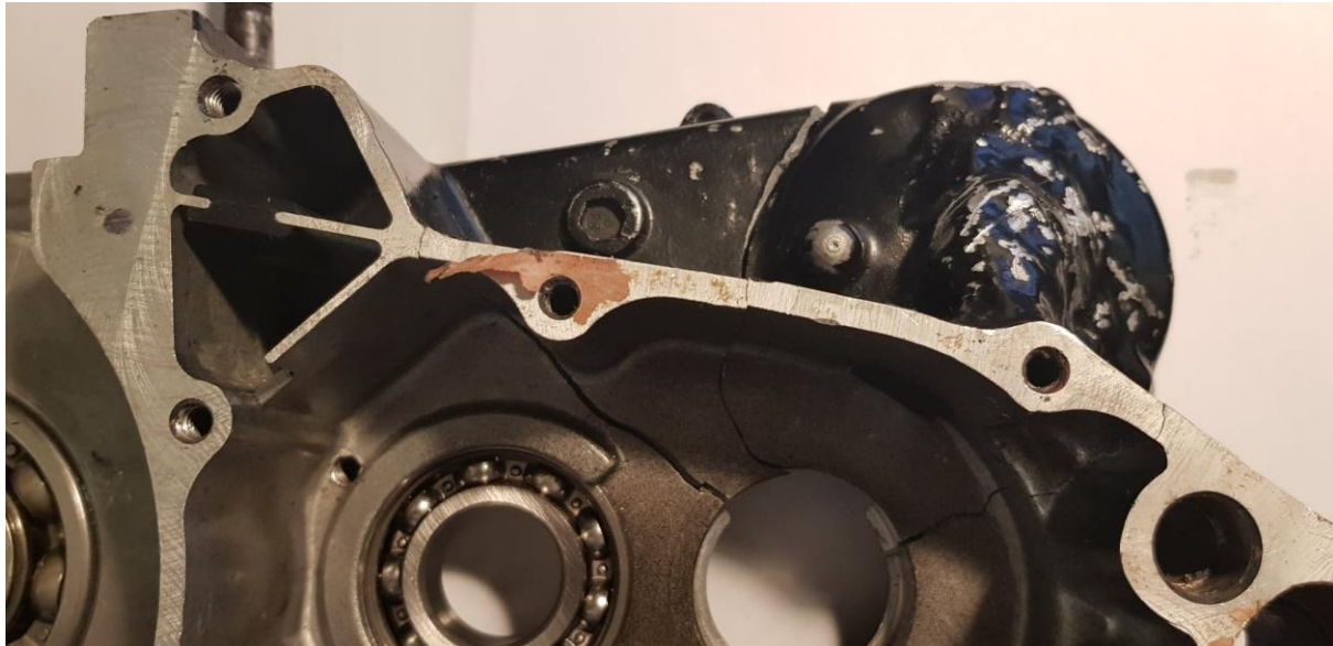
Figure 3 – Right-Hand Crank Case with split around kickstart assembly and output shaft. (Parsons, authors own)
