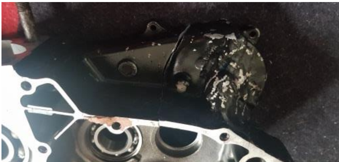
Figure 5 – Right-hand crankcase with crack around kickstart boss. This crank case has been repaired previously. (Parsons, authors own)
