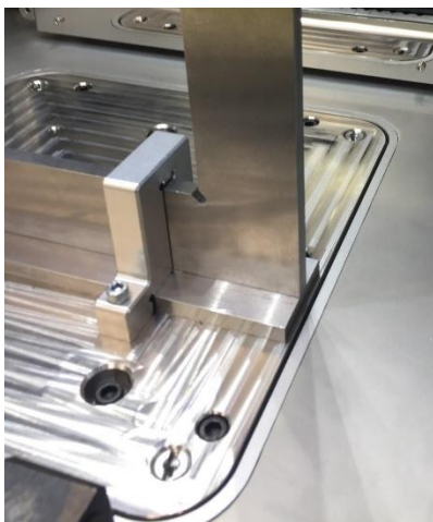
Figure 12 - Clamping Engineers Square
