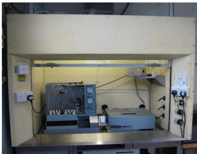
Figure 10. Laboratory automatic sampler and FTIR spectrometer in fume hood.
