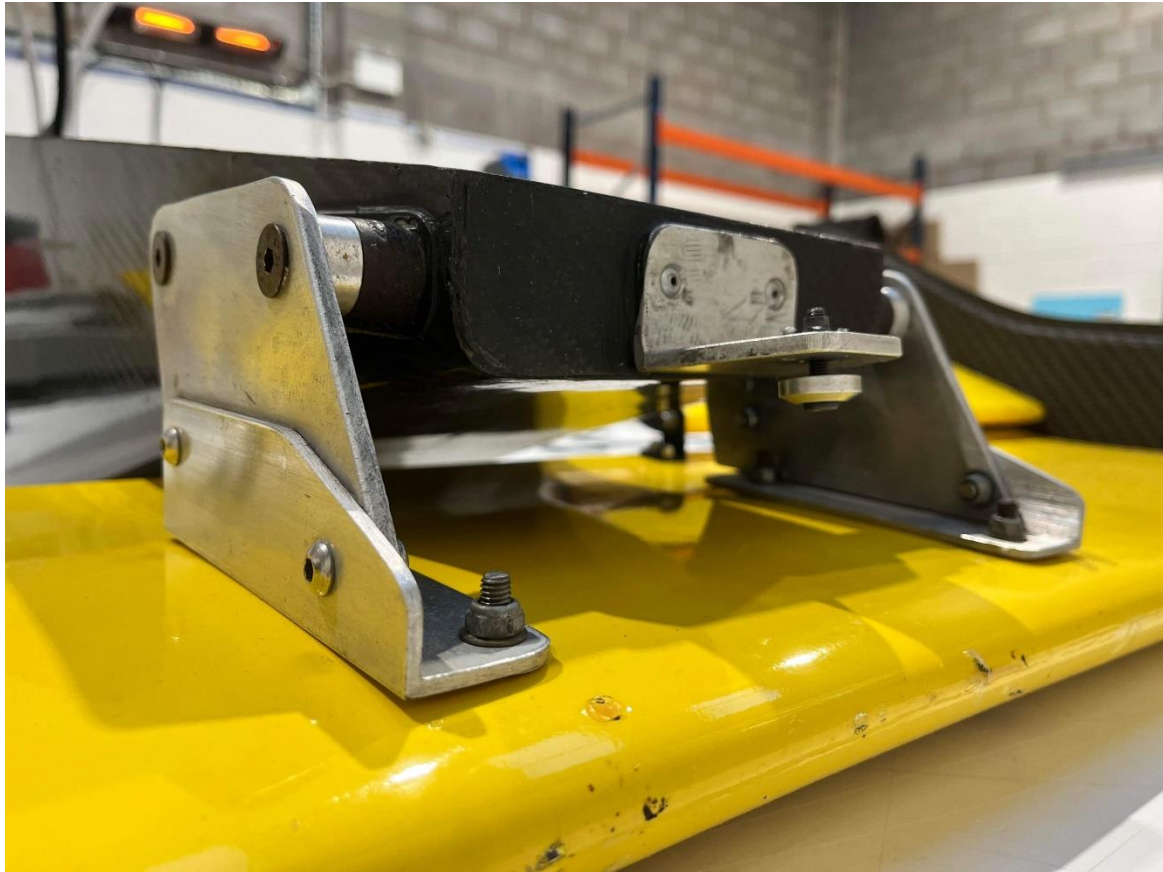
Figure 6 - Front wing mounts of the Force TA (Jones, 2022)
