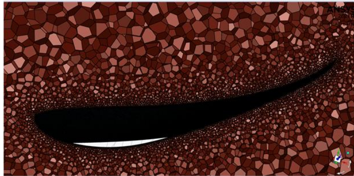
Figure 6 Shows the Polyhedra computed and ready to be solved in Fluent.
