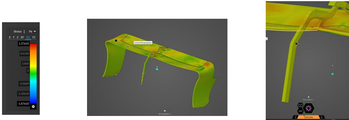
Figure 44 - Initial FEA Simulations Images on ANSYS
