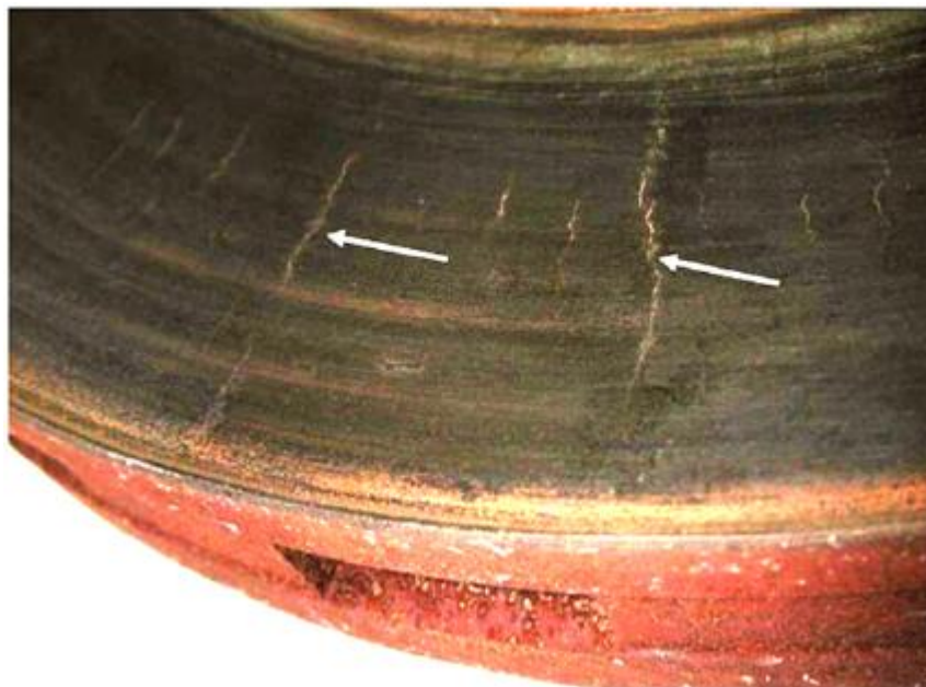
Figure 5 - Cracks in a brake disc caused by thermal stress and fatigue (Lakkam, 2013)
