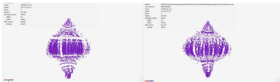
Figure C1 – From L-R test serials 15 and 16 resulting fragmentation
