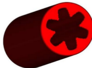
Figure 3 Star grooved propellant [11]
