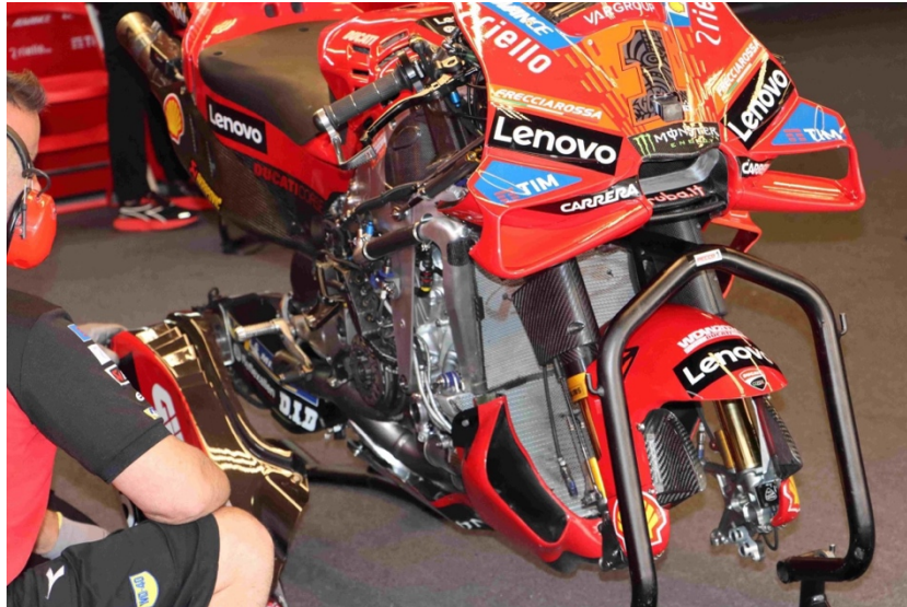
Figure 3 - 2024 Ducati MotoGP Bike, notice the long and thin front engine hanger which is parallel to the centre plane. (Oxley, 2024)
