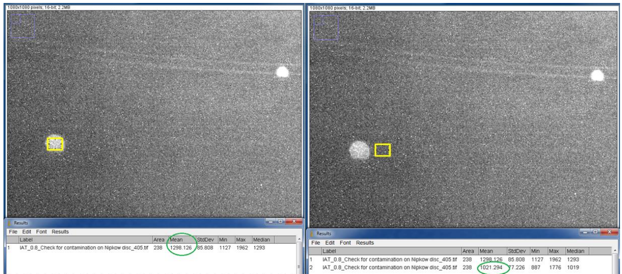
Figure 1-20 - Measuring Bright Spot Mean Intensity
