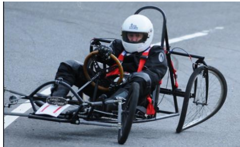
Figure 6 - Gravity racer's wheel buckling from lateral forces (ScottishCarties, 2013).
