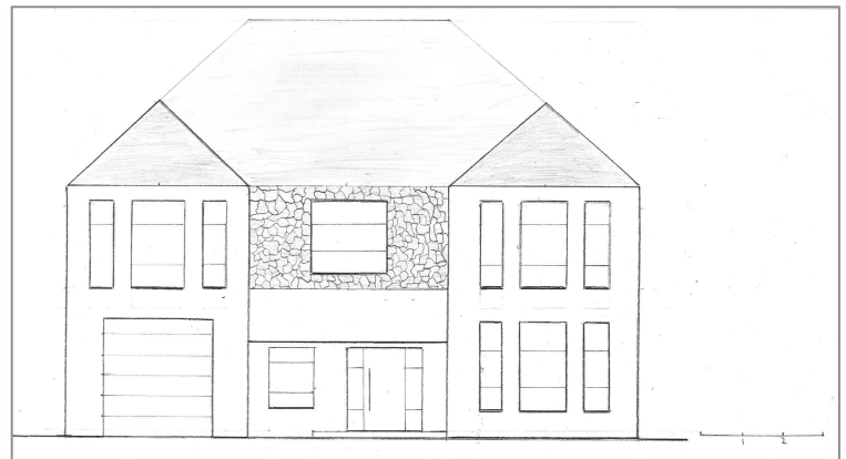
1:50 scale south side elevation drawing of Arnant, showing the Welsh cladding and revised design. (Author, 2020)
