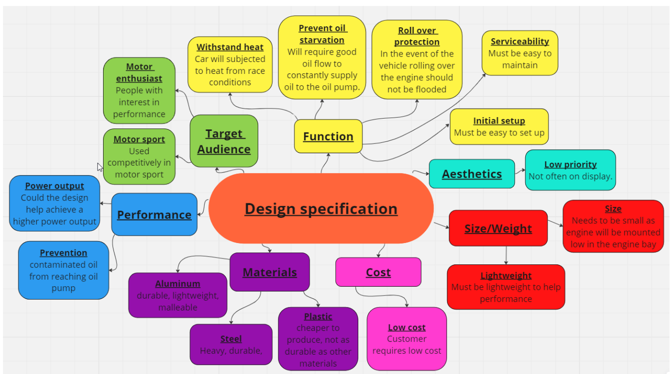
Figure 4-Design specification for the dry sump
