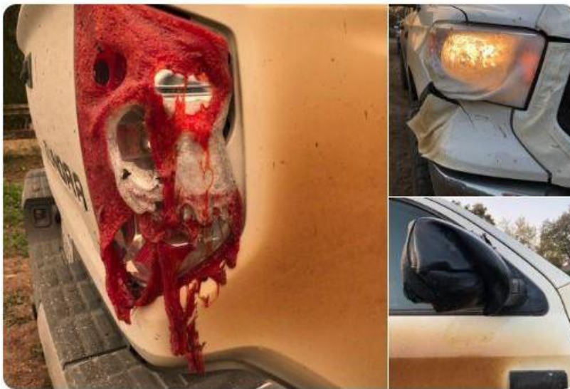
Fig.9 Image of Toyota Tundra showing how it melted in wildfire (Chin, 2019)
