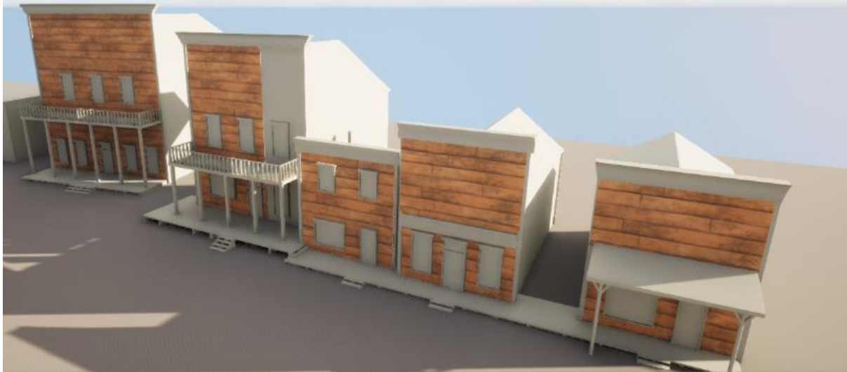
Figure 6.4: UV tiling issue when applying texture to models in Unreal Engine 5
