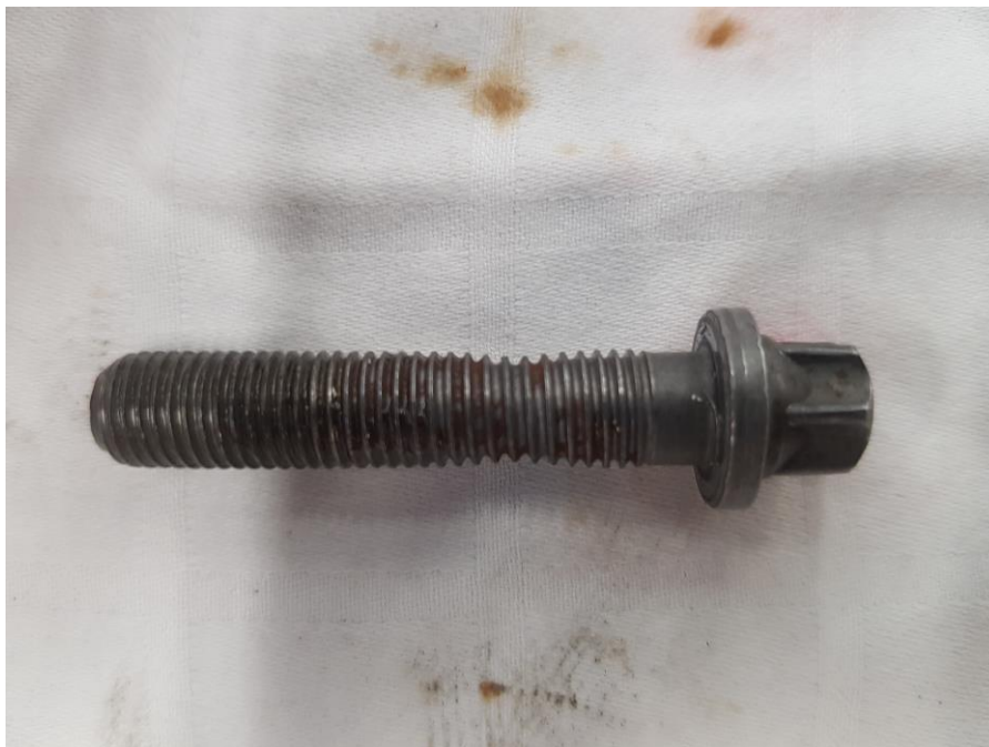
Figure 50 Deformation and stretch of the bolt.
