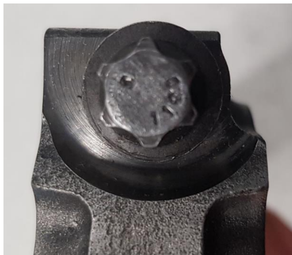
Figure 28 UTS printed on the bolt head.
