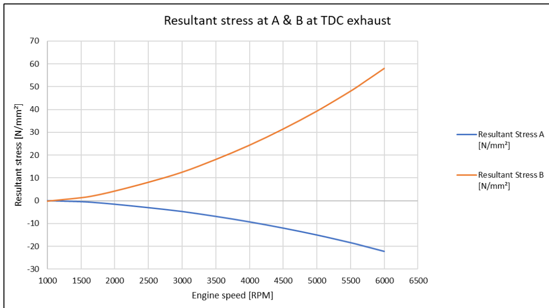
Figure 40 Resultant stresses of A & B at TDC exhaust.
