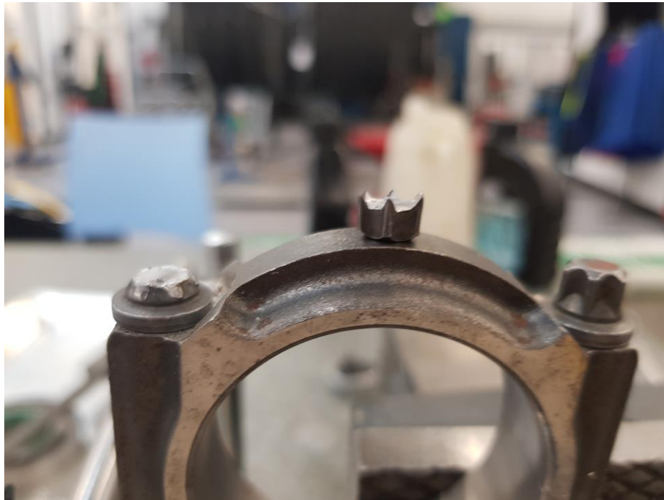
Figure 52 Failed bolt head.
