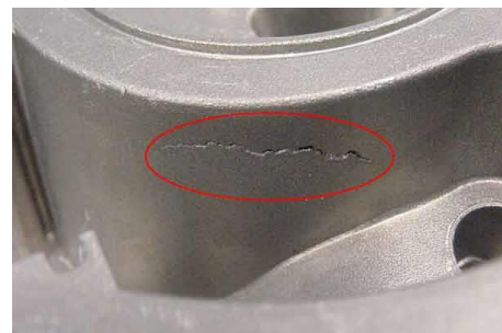
Figure 10: Crack in a die-casted component (Dolin Casting, 2020: Online)
