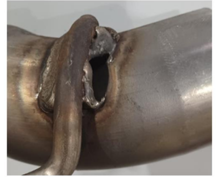
Figure 15: Example of a weld burn-through
