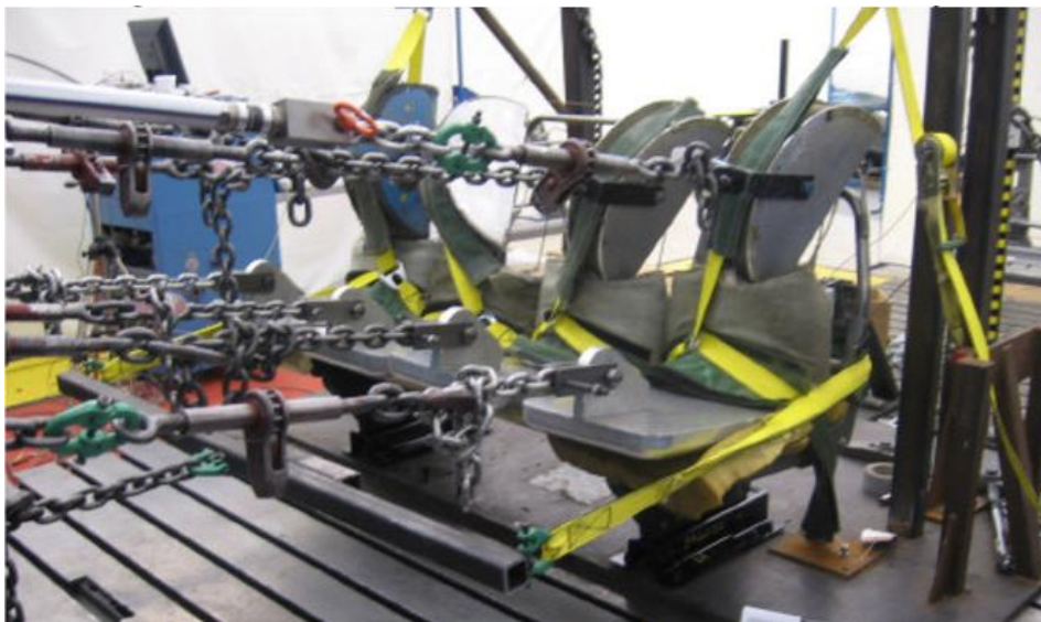
Figure 8 Automotive Seat Structure Test Setup (Radesh Vangipuram, 2008)
