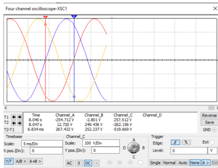
Figure 11- Four channel oscilloscope showing 6.834ms between phases
