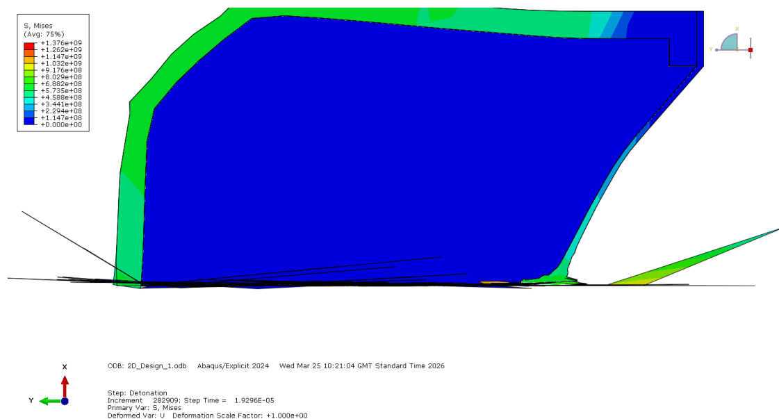
Figure 4: Distortion against the boundary condition
