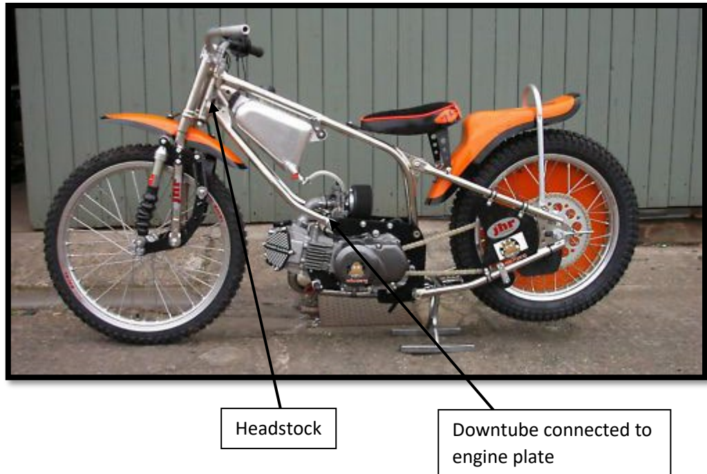
Figure 3 – Labelled Chassis Points on Speedway Motorcycle
