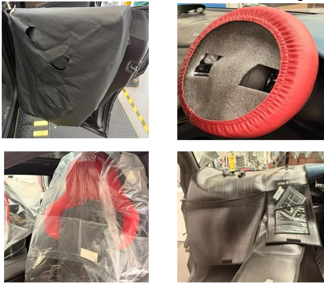
Figure 4 – Examples of temporary protective covers fitted during production
