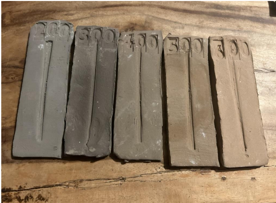
Figure 6: Clay test tiles with temp stamps, own photo (2024)
