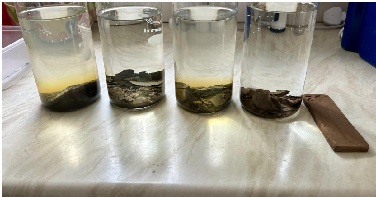
Figure 7: Tests to time how long it takes for clay to break down, own photo (2024)
