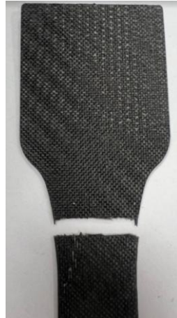
Figure 6 - Carbon Woven Epoxy specimen after failure
