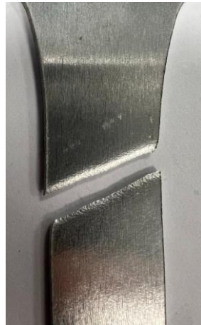
Figure 5 - Aluminium fracture surface showing necking and ductile tearing.
