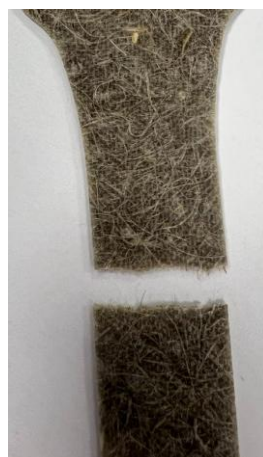
Figure 7 – Flax Non-Woven tear with irregular fibre breakage
