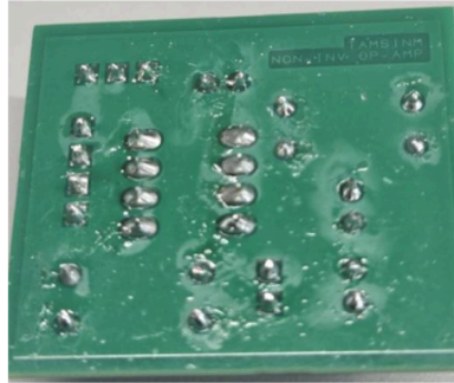
Figure 18: Finished PCB - Bottom
