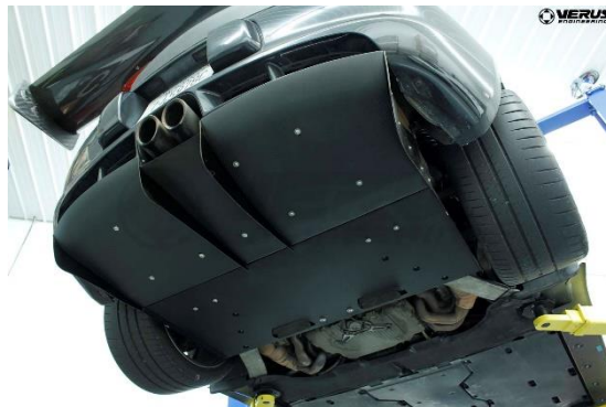
Figure 3 Diffuser with dirty underbody (Verus Engineering ,2019)
