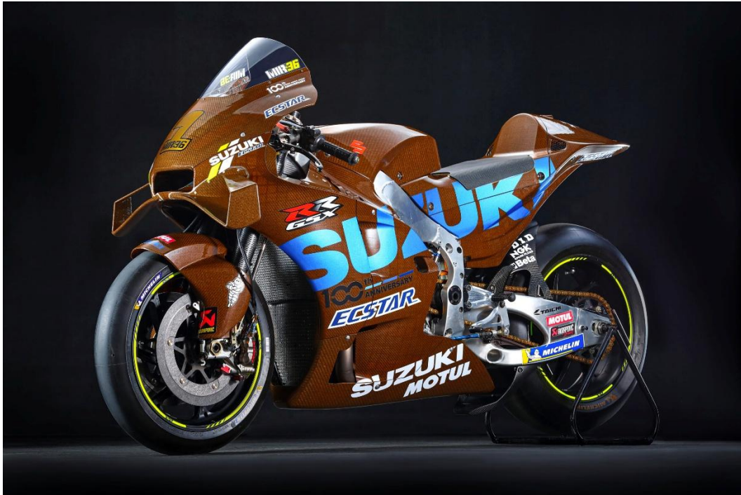
Figure 7: Example of flax-based composite bodywork being explored for use in motorcycle racing (Source: Bcomp, 2025).
