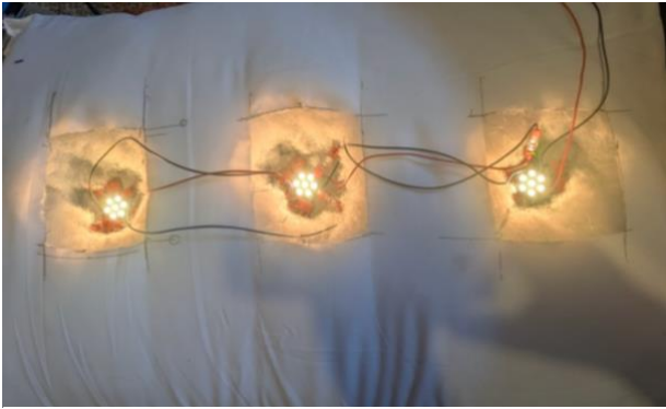
Figure 38: LEDs inserted into cut-out slots in the pillow
