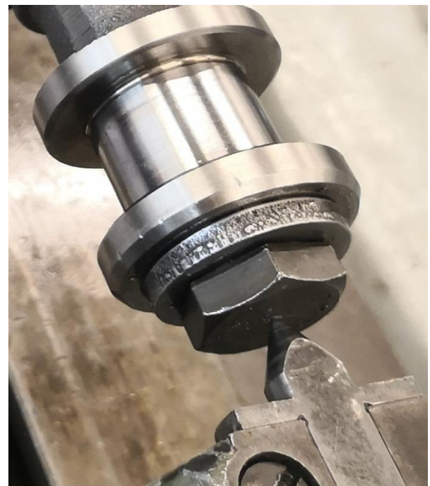
Figures 3.1 Camshaft measuring equipment and final mounting solution.
