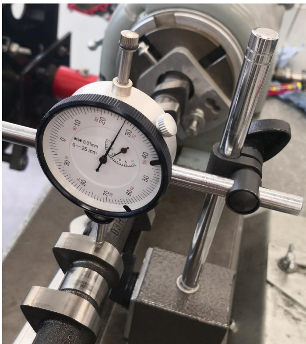
Figures 3.1 Camshaft measuring equipment and final mounting solution.
