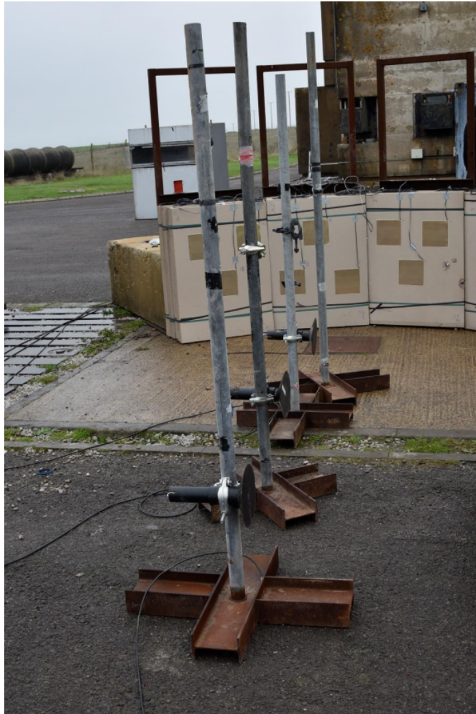
Figure 13: Blast gauges in place.
