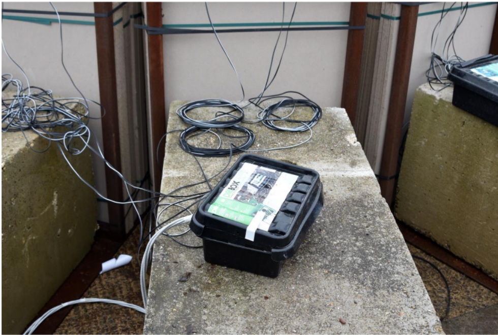
Figure 15: Velocity foil cables and waterproof box used to provide environmental protection to the cable connections.
