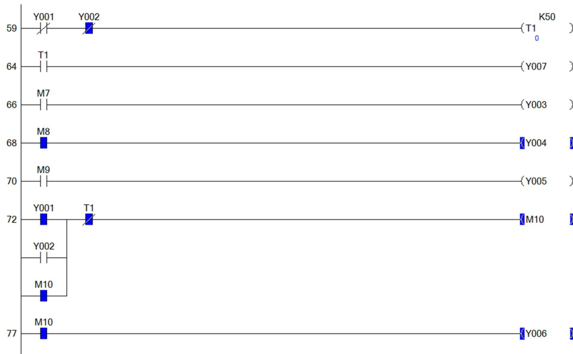
Figure 22 - Lift System Ladder Logic Y006 activated.
