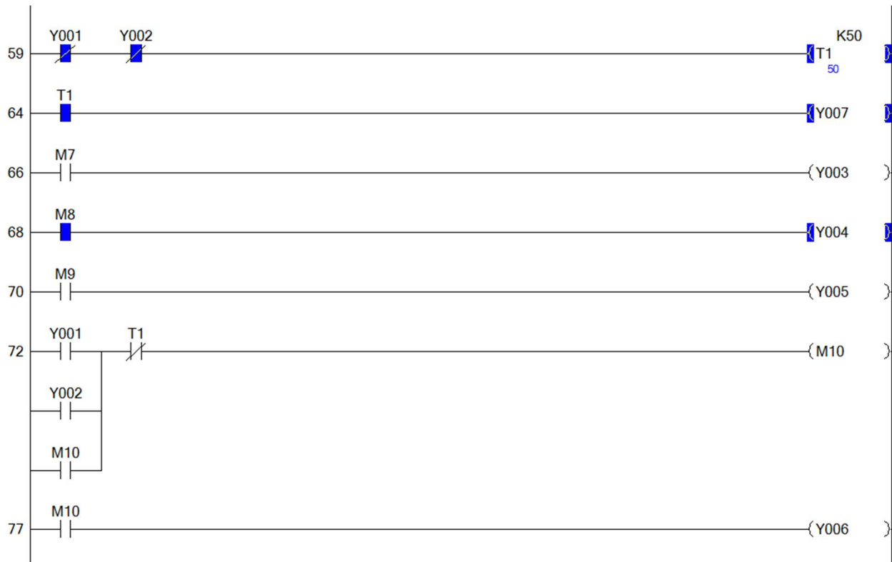
Figure 23 - Lift System Ladder Logic Y006 disengaged.
