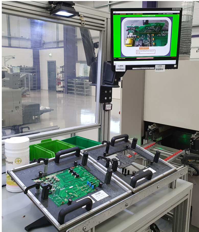
Figure 1. Photo of the through-hole technology component placement station.
