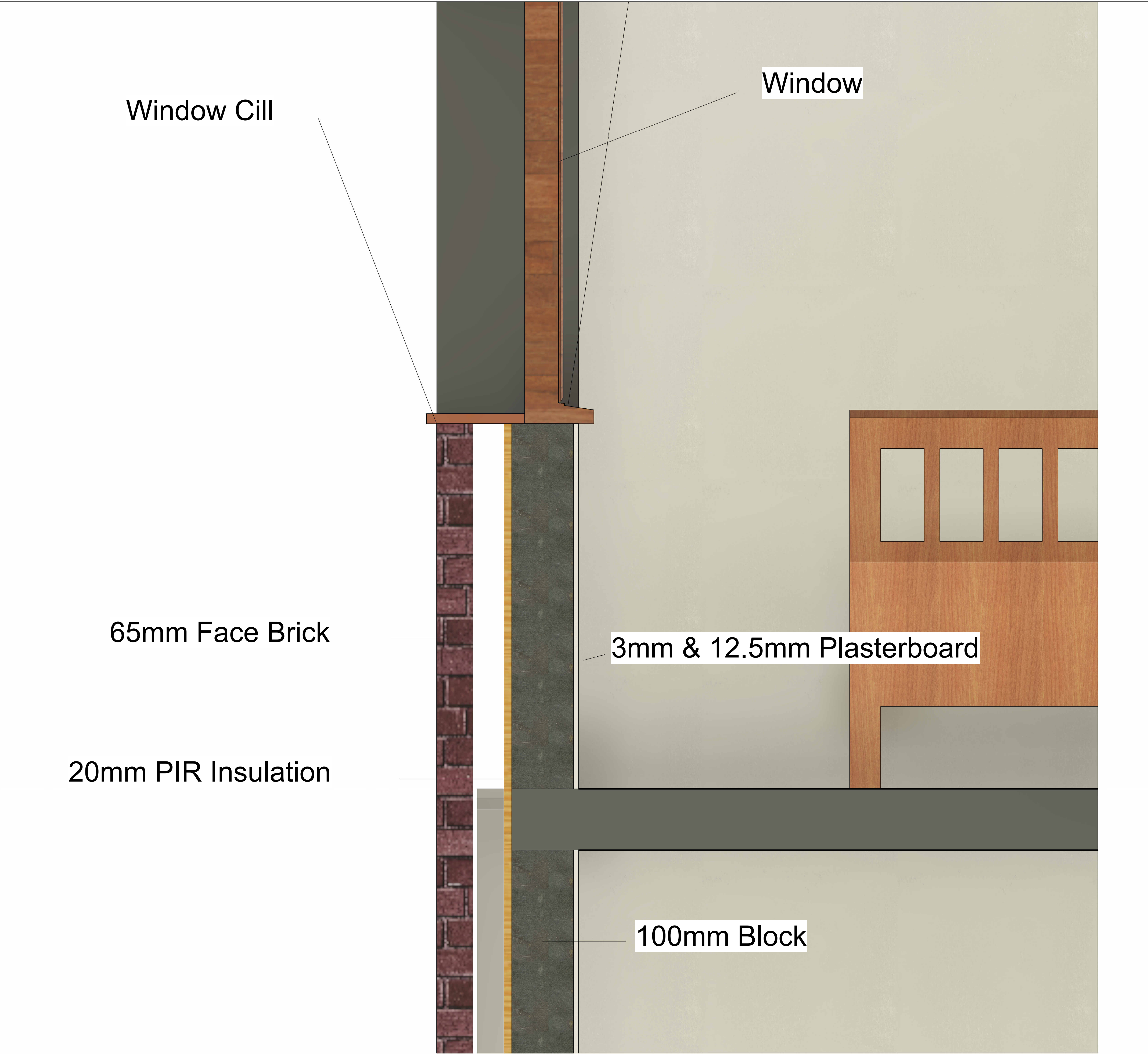
1 Section (3) Call Out Detail 1 : 5
