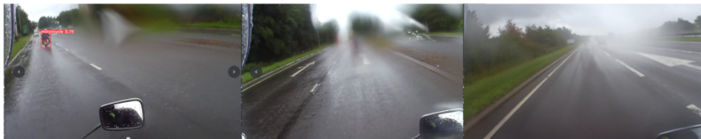
Figure 11.1: Good Detection of Motorcycle - Wet and Multi Lane Figure 11.2: Classification Error - Camera Blinded Figure 11.3: Classification Error - Water Spray from Other Vehicles
