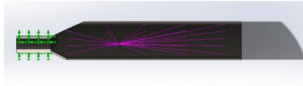
Figure 4 - Centrifugal Force Acting on the Rotor Blade (SolidWorks, 2019)
