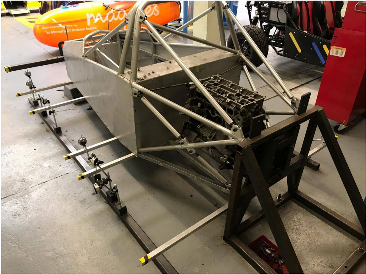
Figure 22 – MCR Chassis mounted to a twist rig, rear view.
