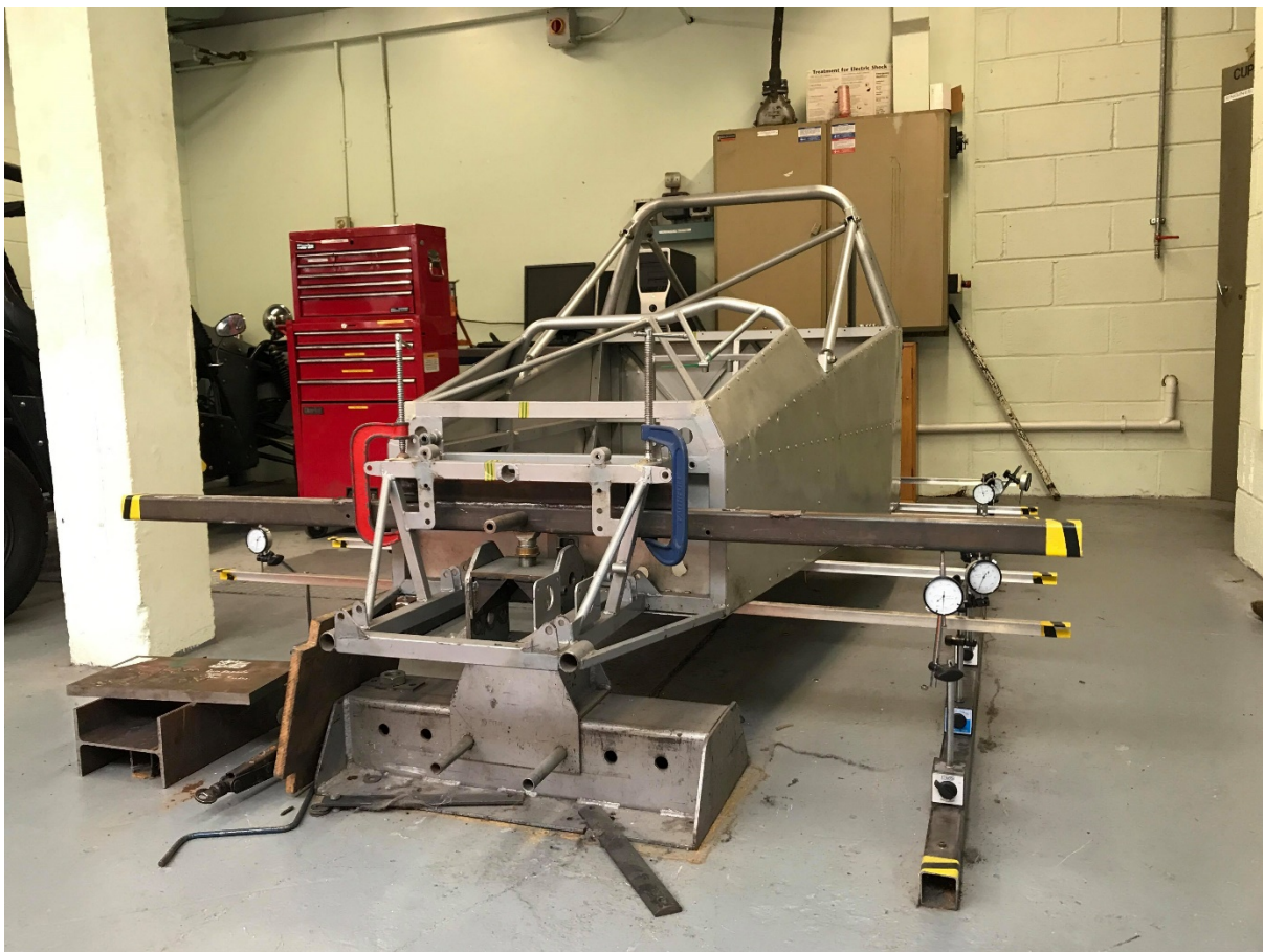
Figure 21 – MCR Chassis mounted to a twist rig, front view.
