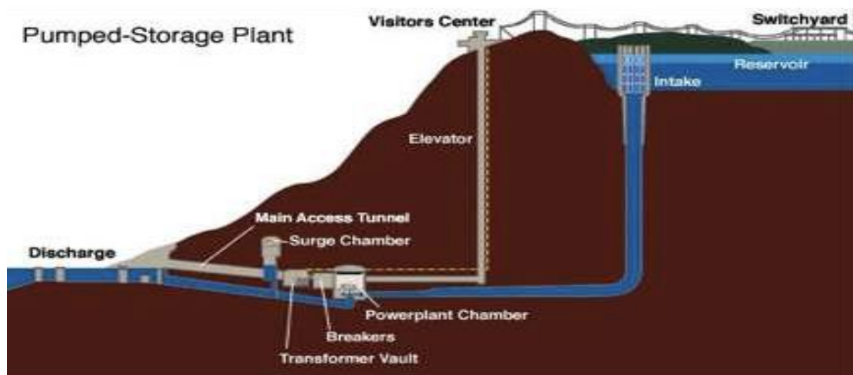
Figure 1. PHS storage plant diagram
