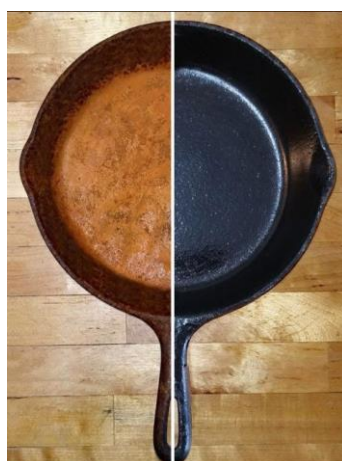
Figure 3 - Corrosion of Cast Iron
