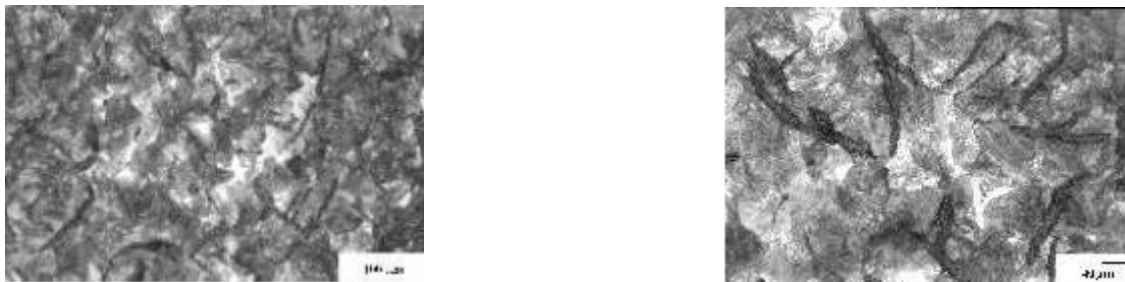
Figure 2 - Microscopic Structure of Grey Iron (Cambridge University, 2001)
