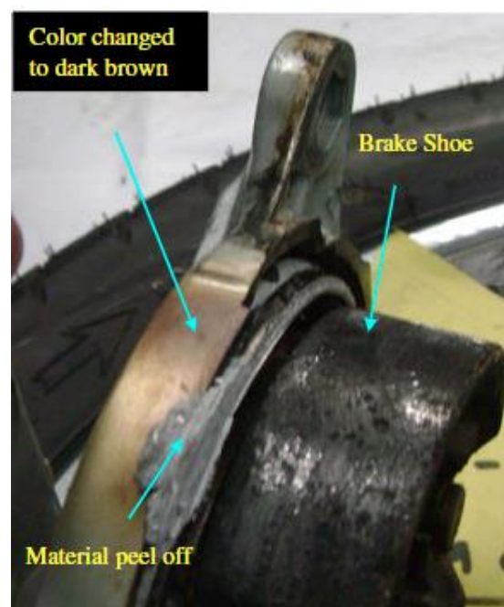
Figure 5 - Seized Drum Brake
